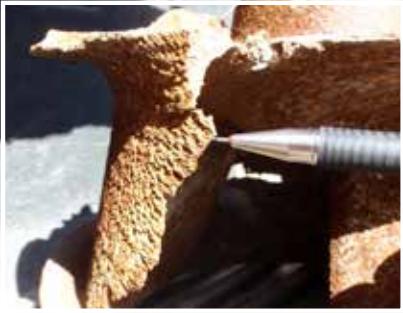
Ashfall will cause accelerated wear and tear on sewage pump impellers (metal pitting and thinning)
