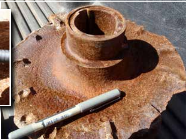
Ashfall will cause accelerated wear and tear on sewage pump impellers (metal pitting and thinning)
